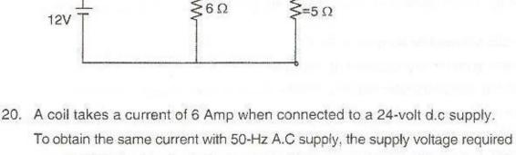
was 30 V. Calculate the inductance and the power factor of the coil.
